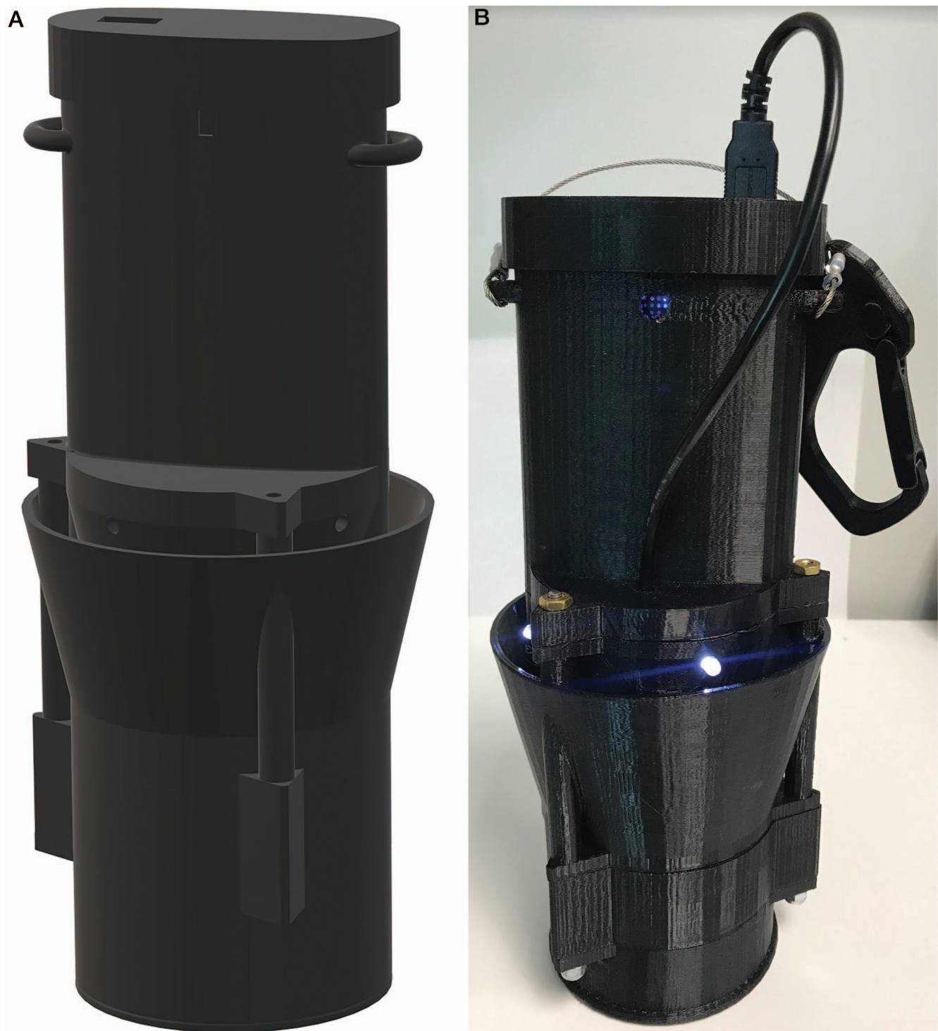
Figure 1.—(A) 3D model of the EVS trap produced using AutoCAD software. (B) Assembled 3D printed EVS trap.
