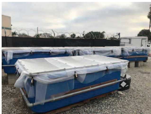
Figure 4. —Arrangement of the large tanks (three treatment tanks and one untreated control tank, foreground) with wood-framed, screened covers.
