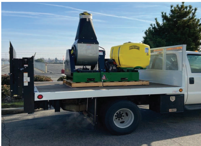
Figure 1. —Picture showing the A-1 turbine and 100 gallon tank on a flatbed truck. This equipment was used for the larviciding treatments using the VectoBac WDG.
