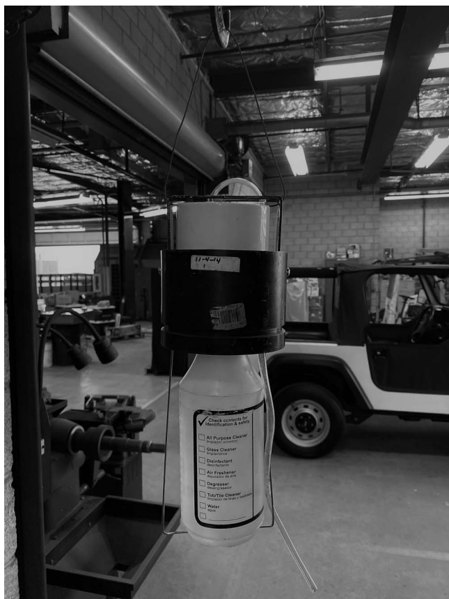
Figure 1. —The Easy Grow: Easy Irrigation System placed inside an old EVS trap casing with a spray bottle screwed to the bottom. A wire supports the bottle.
