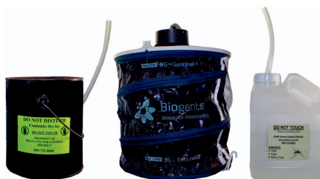
Figure 1.—Dry ice container, BG-Sentinel 2 Trap, and yeast fermentation container.
