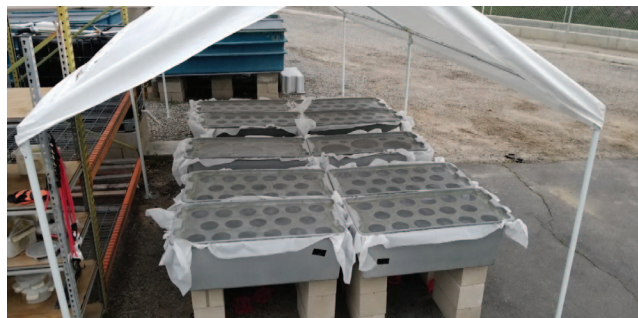
Figure 1.—Arrangement of ten medium-sized tanks (eight treatment tanks and two controls) for testing the efficacy of Sumilarv 0.5G against field and laboratory colony Cx. quinquefasciatus larvae.
