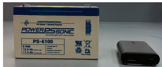
Figure 1.—Comparison of the 6V battery on the left (PowerSonic PS-6100) and the lithium-ion battery on the right (Anker A1263).
