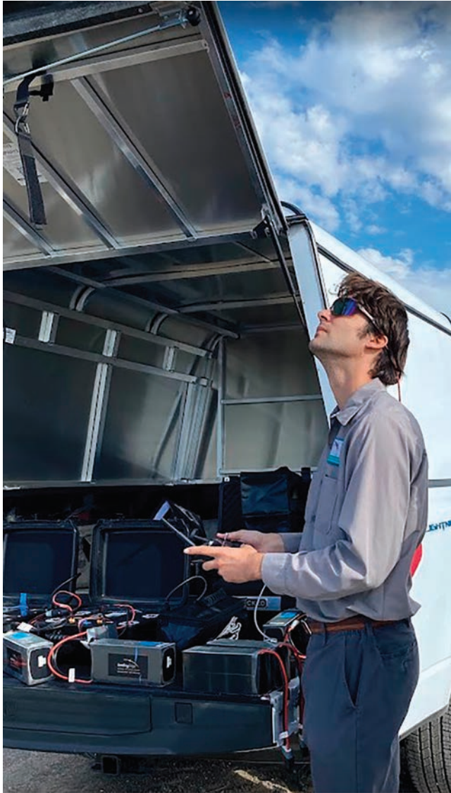
Figure 3. —Drone batteries charging efficiently from the Ford F-150 Lightning's Pro Power Onboard system.
