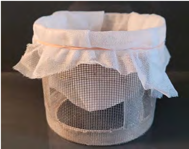
Figure 1. —Larval sentinel cage made from a modified BioQuip emergence cage bottom, with polyester mesh liner held in place by a rubber band.
