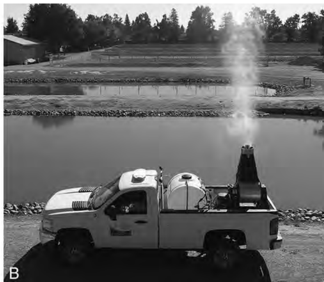
Figure 1. —A) A1 SuperDuty A1 fan air driven mist sprayer – Manufacturer Photo. B) A1 SuperDuty Mist Blower modified and mounted on District Truck.
