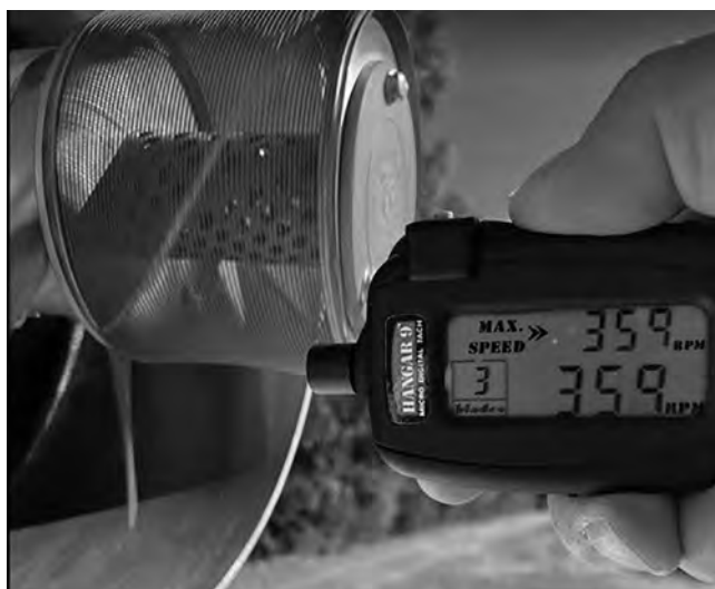
Figure 3.—RPM meter positioned in front of spinning Micronair Rotary Atomizer.
