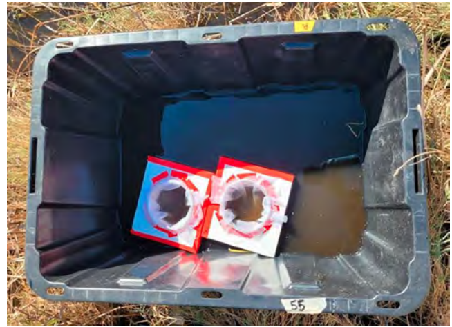
Figure 2. —102-liter (27-gallon) bin holding pond water and two floating sentinel cages, each containing 15 lab-reared Culex tarsalis larvae.
