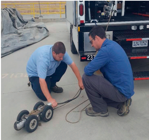
Figure 3. —Remotely-powered rover with closed-circuit TV used for inspection of sewer systems.
