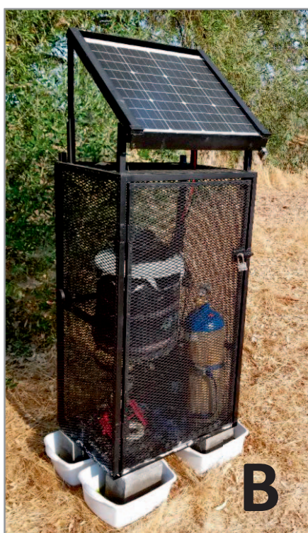
Figure 1. —a) BG Counter automated mosquito counting device. This device is designed to sit atop a BG Sentinel mosquito trap and count mosquitoes entering through the central opening using infrared sensors. Data are transmitted with a cellular data connection. b) A BG Counter deployed in the field, with BG Sentinel trap, battery, CO 2 supply, solar panel, and welded enclosure
