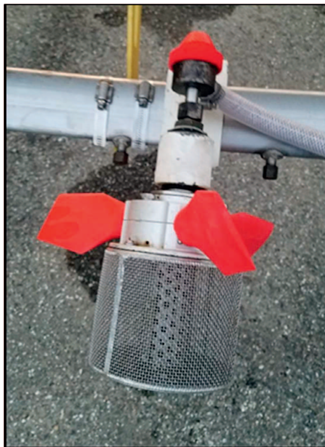
Figure 1.—Rotary Atomizer (Micronair AU5000®) showing the mesh cage and fan blades
