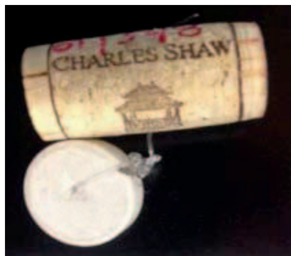
Figure 1. —A Natular T30 tablet that is tied to a wine cork by a piece of Nylon fishing line.
