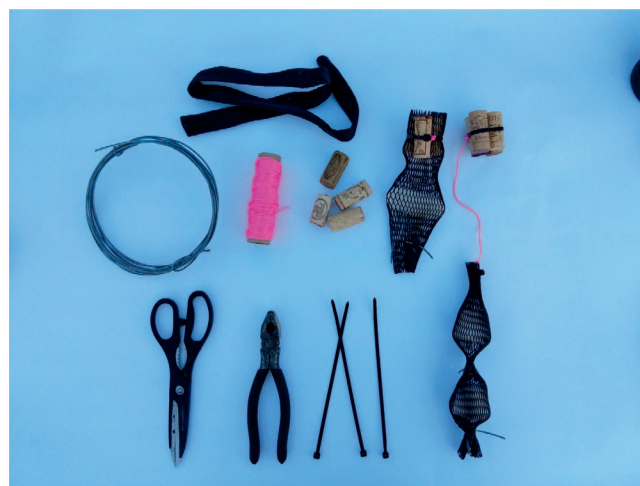
Figure 1.—Materials used to construct floatation device for long term larvicide products.
