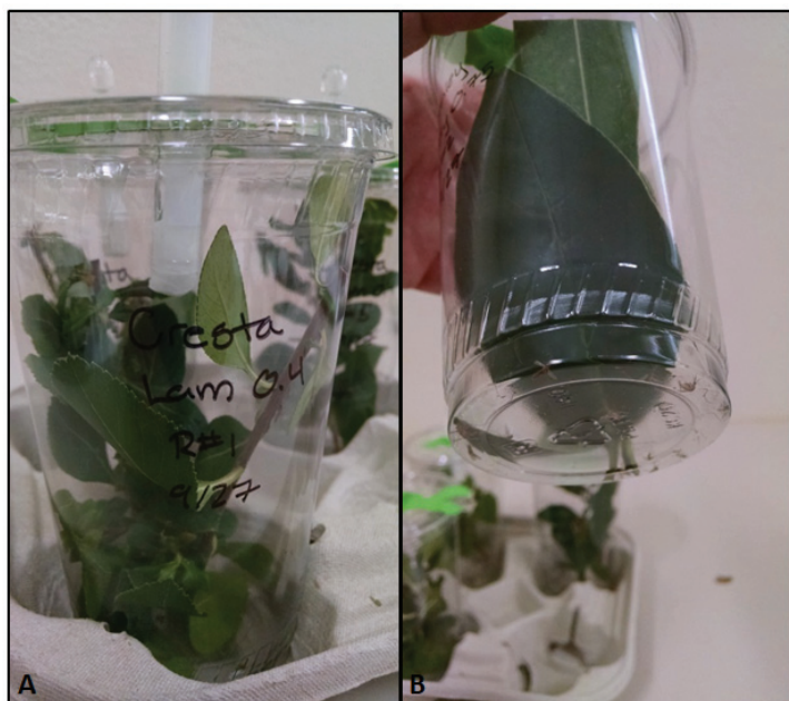
Figure 2 Leaf bioassay cups. Panel A shows the complete cup set-up with a sugar wick placed in the straw opening of the lid. Panel B shows dead mosquitoes in the bottom of assay cup that were counted to calculate percent mortality.
