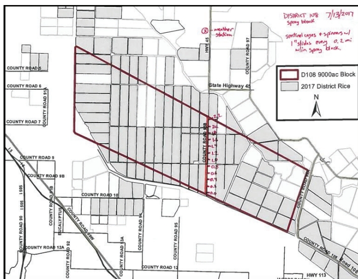
Figure 1 A typical layout of sentinel cage and droplet spinner sites in an aerial spray block (District 108 in Yolo County).
