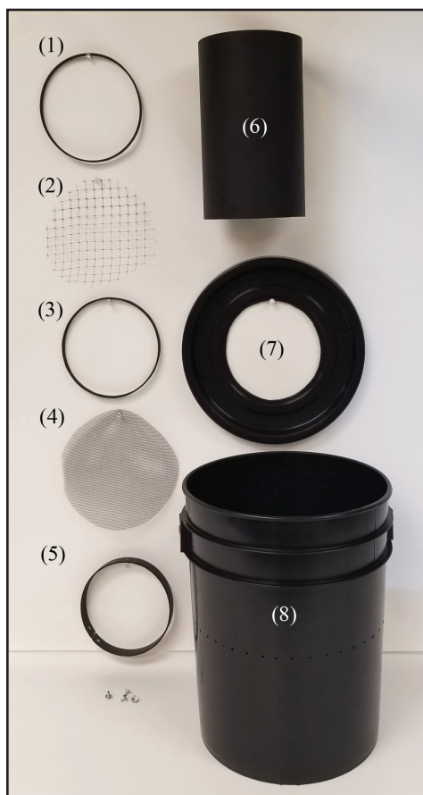
Figure 1 The trap was made with a black 5-gallon bucket (8) with a lid (7). To create the resting and capture arena, a 10" length of a 6" diameter PVC pipe was used (6). To hold fabric in place, rings were cut from a separate 6" diameter PVC pipe in 1/4" (1 and 3) and 1/2" lengths (5). A 1-in section was removed from the 1/2" rings. The rings were heated in an oven at 392°F until softened to allow for stretching around the 6" PVC pipe perimeter. Fiberglass window screen was added to one end (4 – held in place with the 1/2" ring), and 1/2" bird netting was added to the opposite end of the pipe (2 – held in place with the 1/4" rings). All PVC pipe pieces were painted matte black.
