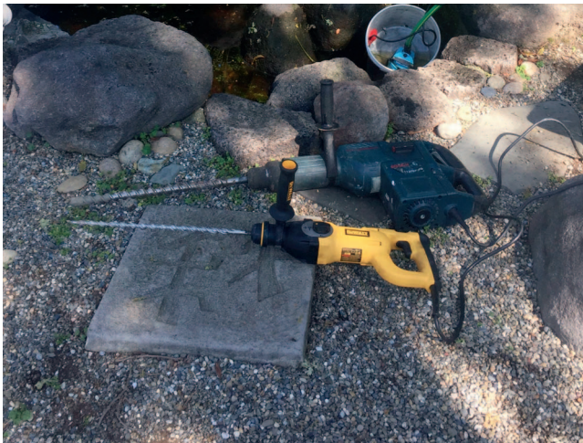
Figure 3. —Two commonly used types of impact drills for pond drainage: shown are a Bosch 11245EVS with a 1-1/8" drill bit and a Dewalt D25231 with a 1" drill bit.
