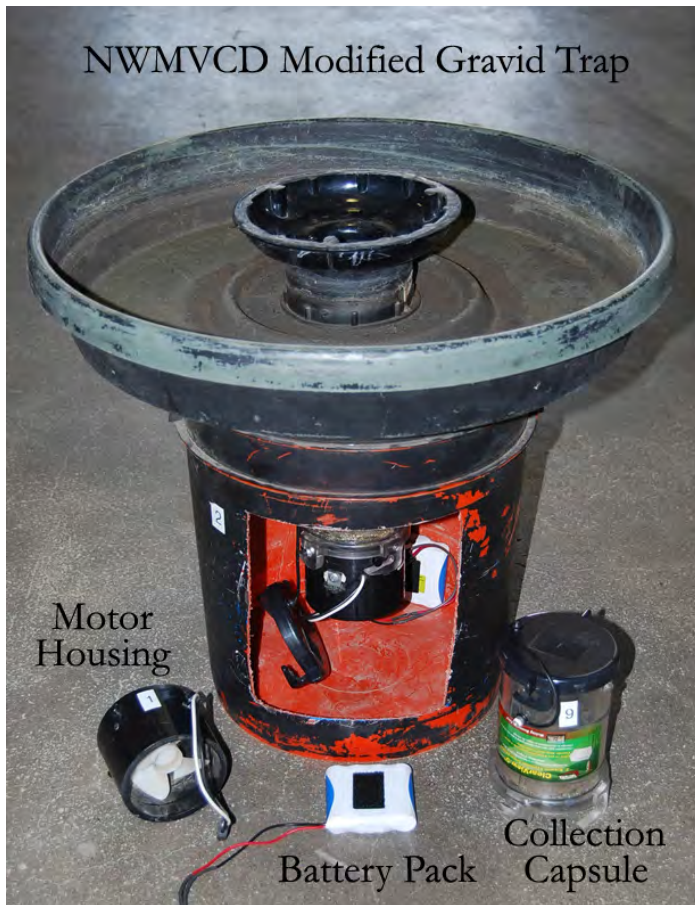
Figure 1. In-house modified down draft gravid trap and components: Collection capsule is placed underneath reservoir dish (where the gravid attractant is placed) with center piece removed (5-inch diameter hole) and replaced with ABS cuff and clip for capsule attachment, inside of 5-gallon bucket. This cuff is conduit for air flow and functions to keep the gravid attractant contained. The bucket has an 8 x 8 in 2 hole on one side to allow access to the clip and cuff. The collection housing has pegs that lock into the cuff clips. The motor capsule attaches in the same fashion and contains a battery lead for the Lithium ion battery pack.
