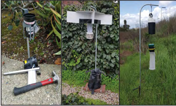
Figure 1. Ovi-cup support (left), on-ground support with suspended Faye-Prince Trap (center), and in-ground support with suspended CDC EVS CO 2 trap (right).
