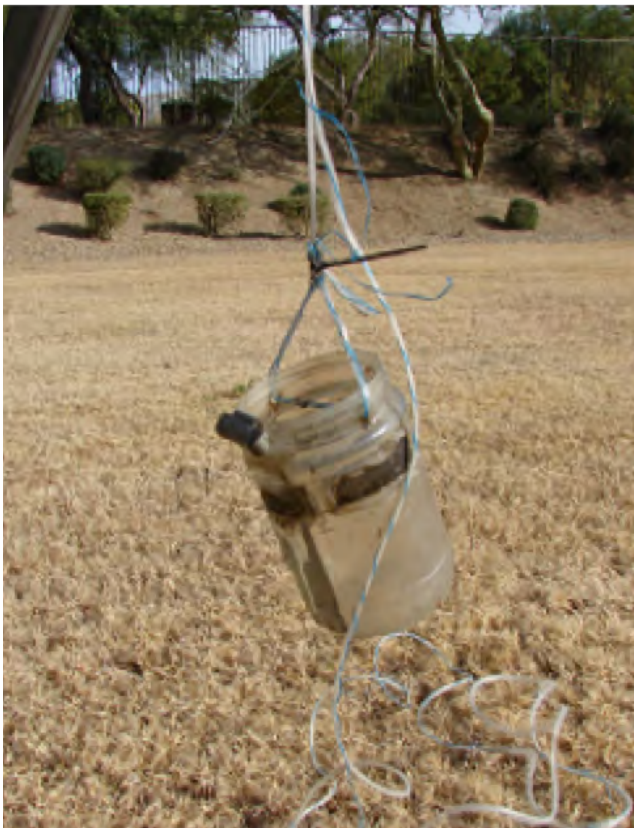
Figure 3. Modified dipper. The nylon rope allowed the dipper to be lowered to the appropriate depth, and the lead weight kept the opening down while the cup filled with water.
