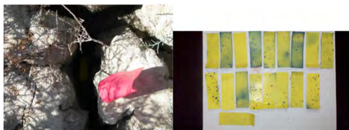
Figure 1. Water sensitive cards. Placement in the field (left) and after treatment (right).
