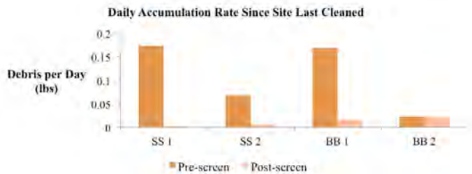
Figure 4. Daily accumulation rates of debris before and after screens.
