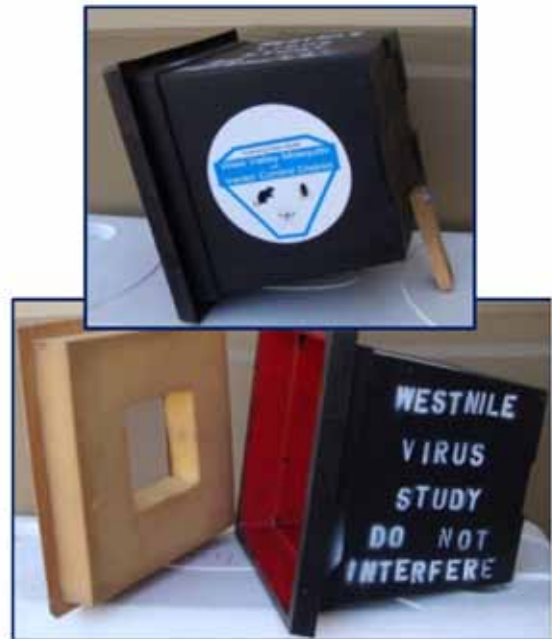
Figure 1. Construction of the mini resting box.
